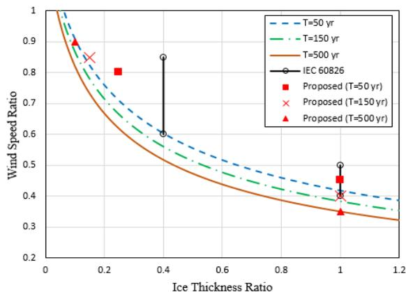
Fig. 3. Proposed reduction factors compared to 84% hazard curves and IEC 60826 factors
