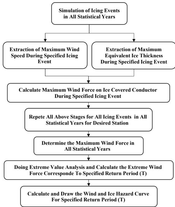
Fig. 1. Process of preparing ice and wind hazard curves for a typical meteorological station
