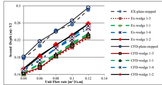
Fig. 7. Numerical and laboratory secondary water depth of a simple stepped spillway and stepped spillway with a wedge element type 1.
