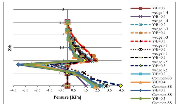
Fig. 5. Vertical profile of the Pressure distribution in the vertical wall at  $x = 0$  ( $Z$  is the distance from the floor of the step and  $h$  is the height of the step).
