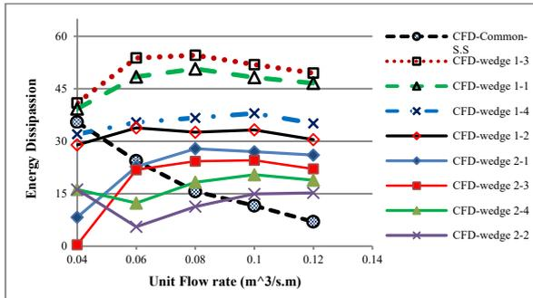
Fig. 3. Energy dissipation for simple stepped spillway and stepped spillway with wedge elements.
