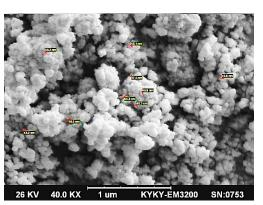
Figure 1. SEM image of zinc oxide nanoparticles
