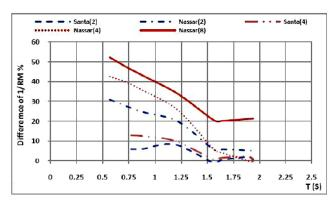
Fig. 2. Comparison of ductility modification factor  $(1/R_M)$  for near fault ground motion proposed in this study with those in previous investigation for far fault ground motions [2,6].
