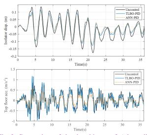
Fig. 2. Comparison of the time history of a) base displacement and b) roof acceleration under the Hachinho earthquake record
