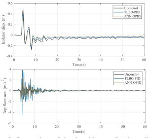
Fig. 3. Comparison of the time history of a) base displacement and b) roof acceleration under the Northridge earthquake record
