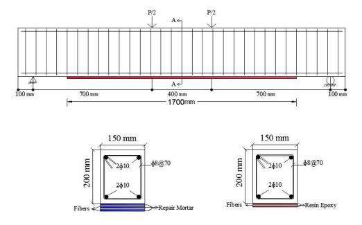
Fig. 2. The dimension, longitudinal and transverse reinforcement arrangement and the location of the applied loads (the dimensions are based on mm) of (a) the specimen strengthened with CFRP and epoxy resin and (b) the specimen strengthened with CFRP and cement-based mortar
