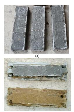
(b) Fig. 1. Poured cement-based mortars in (a) compressive strength test form and (b) tensile strength test form
