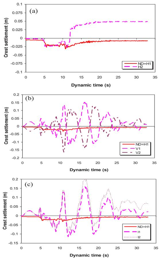
**Fig. 2. Time-history response of the crest settlement under irregular seismic loadings in the direction of: (a) horizontal, (b) vertical, (c) inclined**
