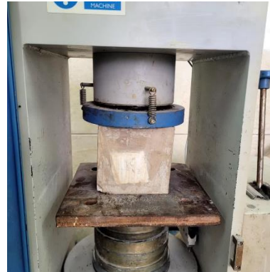
Figure 16. a) Compressive strength fracture test of cubic specimen with concrete breaker jack b) Broken specimen of self-compacting concrete with fiber and iron oxide.
