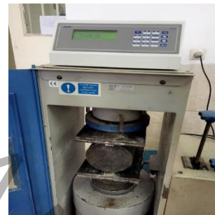
Figure 17. a) Tensile fracture test of a cylindrical specimen with a concrete breaker jack b) Broken specimen of self-compacting concrete with fibers and iron oxide.
